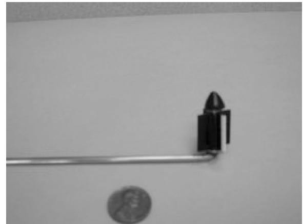
Fig. 11 Simple vorticity meter.
